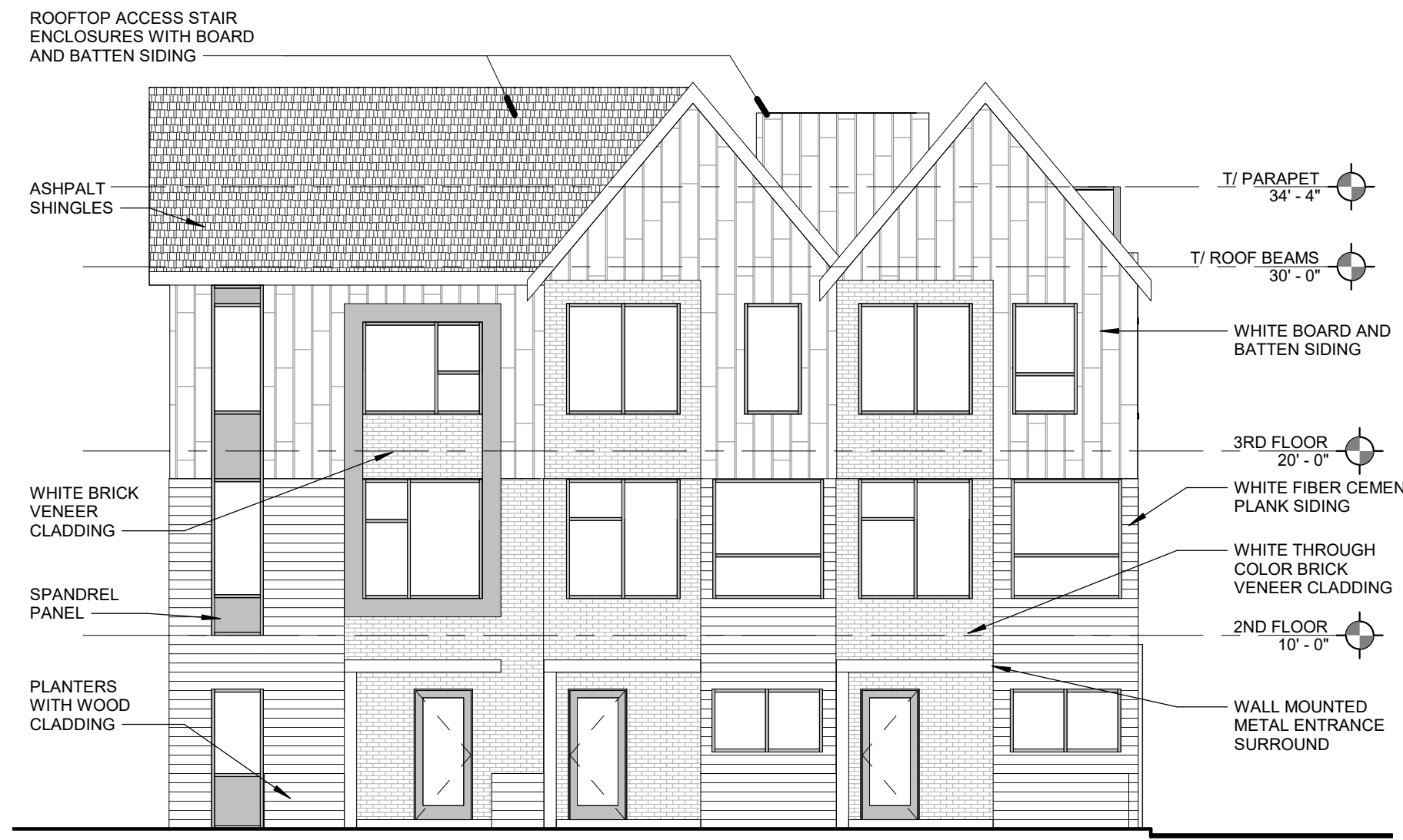
5 SOUTH BUILDING ELEVATIONS, FACING MOLER SCALE: 1/8" = 1'-0"
