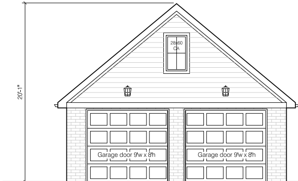
GARAGE SOUTH ELEVATION
