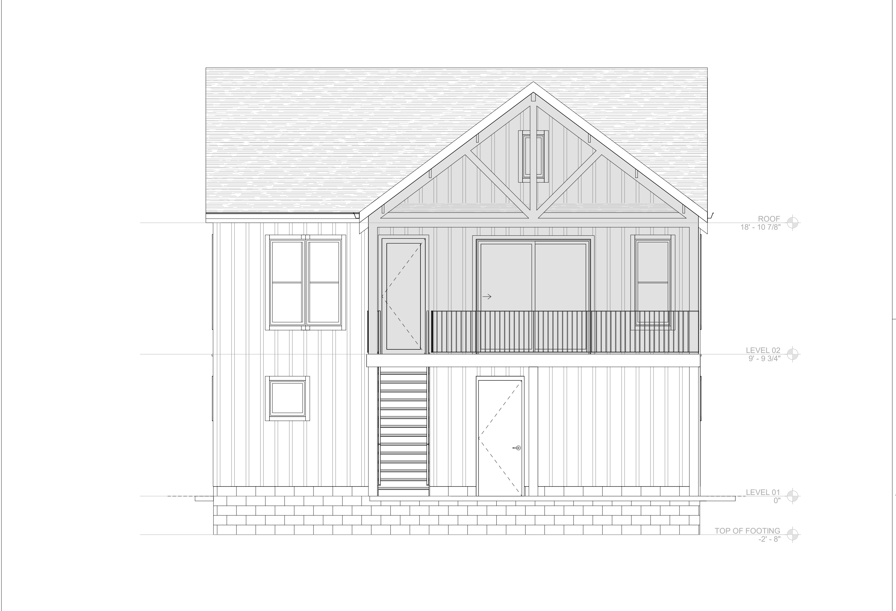
A2 EXTERIOR ELEVATION - SOUTH G03 SCALE : 1/4" = 1'-0"
