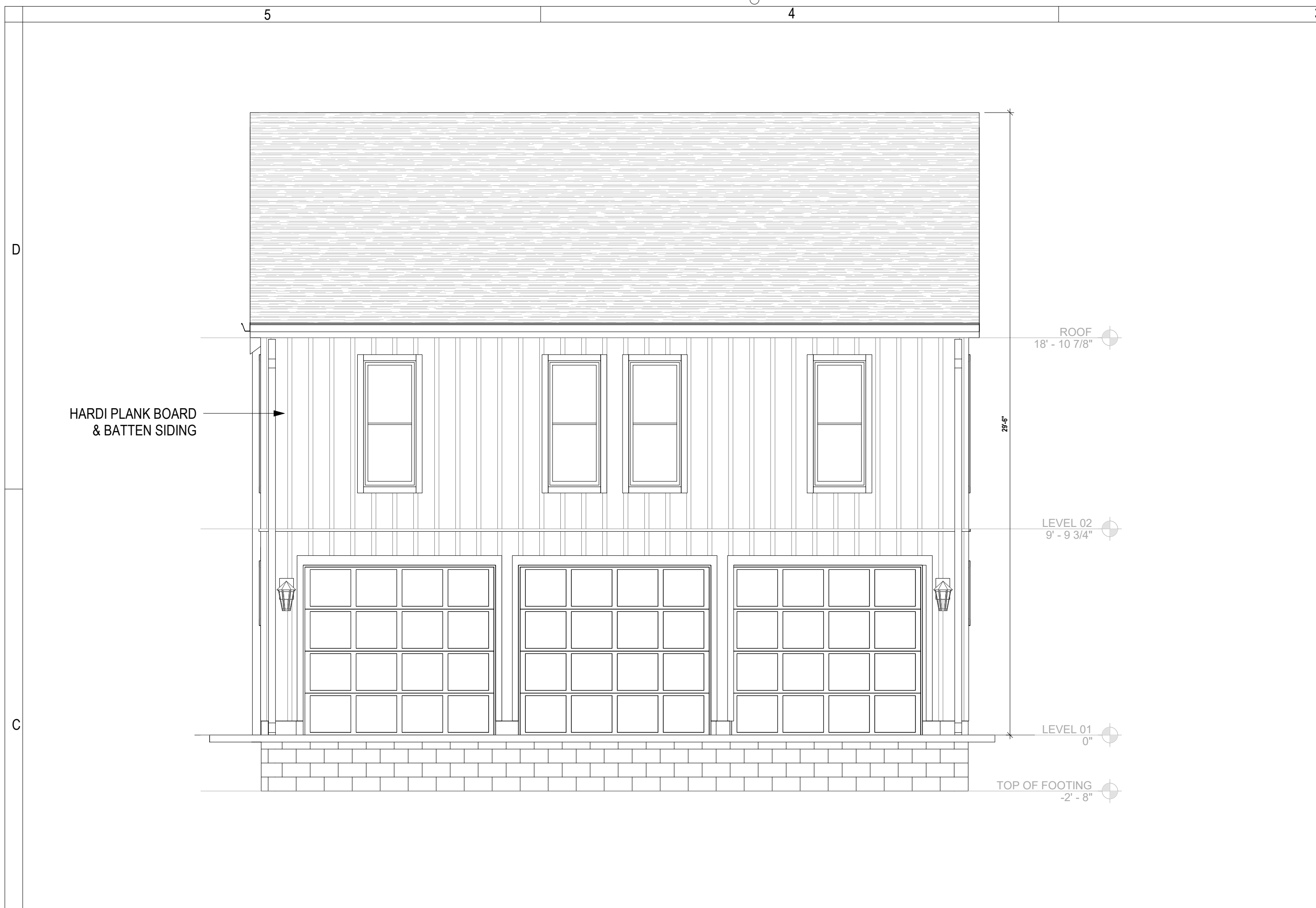
C5 EXTERIOR ELEVATION - NORTH G03 SCALE : 1/4" = 1'-0"
